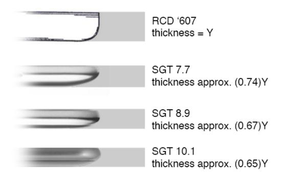
By contrast with the crisp edge of the design, all three of the Samsung products have a side which curves a little <u>outwards</u> (so a bit bezel-like) before curving back in and under. And none of them have a vertical portion.
