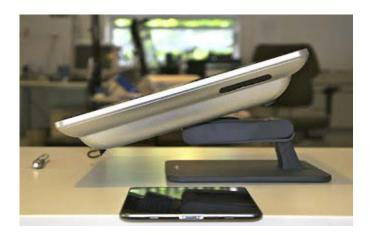
The stand (shown in dark grey) could be optionally fitted to the silvered computer which could be hand-held. So it is irrelevant. But the lump on the back of the screen was integral with it. No doubt it contained functional electronics and the like. We were shown a physical example of the Flatron – it is much bigger than any of the Samsung products (or an iPad for that matter). Just about hand-holdable.
